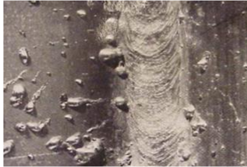
Fig. 3.2.10. Visual characteristics of spatter. Source: M.S. Rogers, Welding Inspection Defects/Repairs Course Reference WIS 5, 2003.
