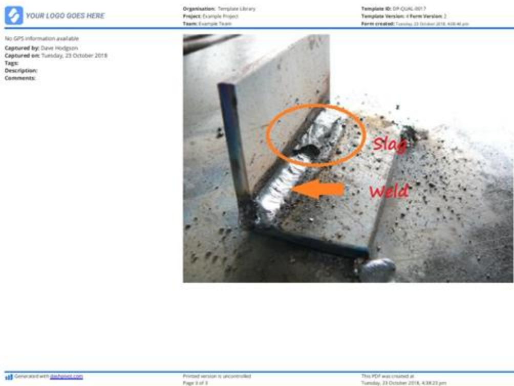
Fig. 3.2.36: Documentation practice example 3/3. Source: https://sitemate.com/templates/quality/forms/visual-weld-inspection-template/
