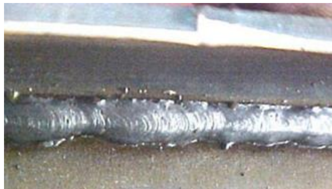
Fig. 3.2.30: Incomplete penetration. Source: https://allgas.us/b/what-are-welding-defects--types-causes-and-remedies
