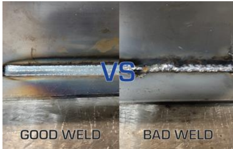
Fig. 3.2.33: Difference between good and bad weld, example 2. Source: https://blog.daihen-usa.com/why-welding-parameters-are-so-important-to-finished-quality
