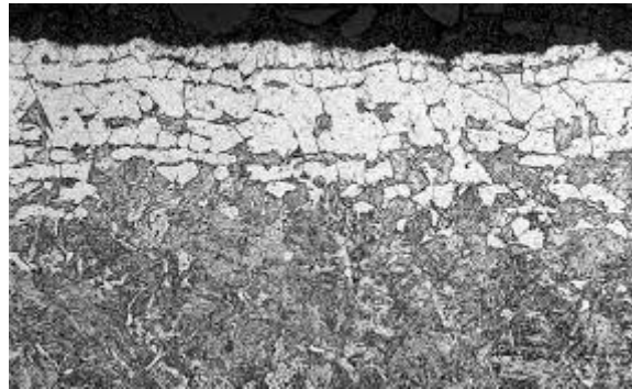
Figure 3.6.3. Decarbonized surface of C-Mn steel
