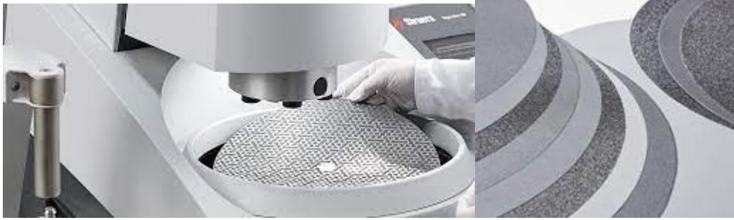
Figure 2.2.37. Grinding and polishing machines or equipment, abrasive papers (source: Kemet International Ltd)
