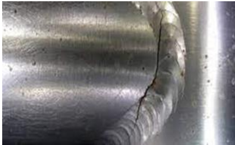
Fig. 3.2.28: Crack. Source: https://www.rapidirect.com/blog/types-of-welding-defects/
