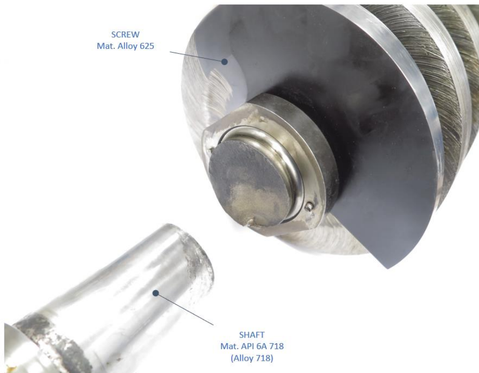
Fig. 2.6.5 – Example of nickel alloy shaft fractured by fatigue phenomena. Source: IIS Laboratory.
