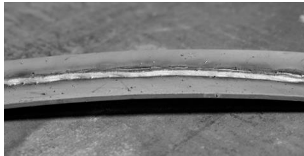
Fig. 1.3.20.2: An example of distortion [1.3.31]
