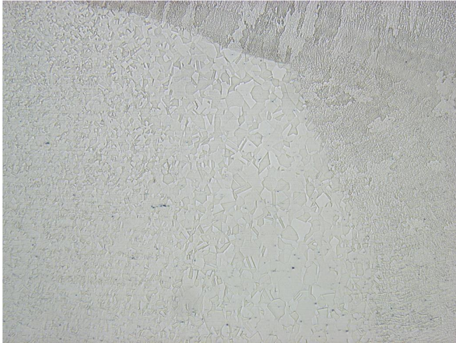
Fig. 3.5.10 – Heat affected zone (HAZ) of austenitic stainless-steel type AISI 316 (25 x). Coarsened grains in HAZ.
