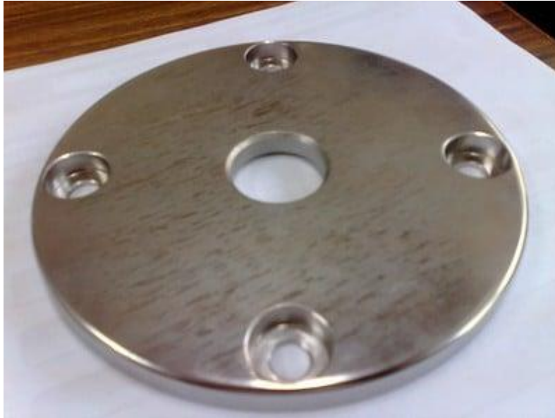
Figure 2.2.19. Streaks on machined SS304 after electropolishing (source: Global Spec)
