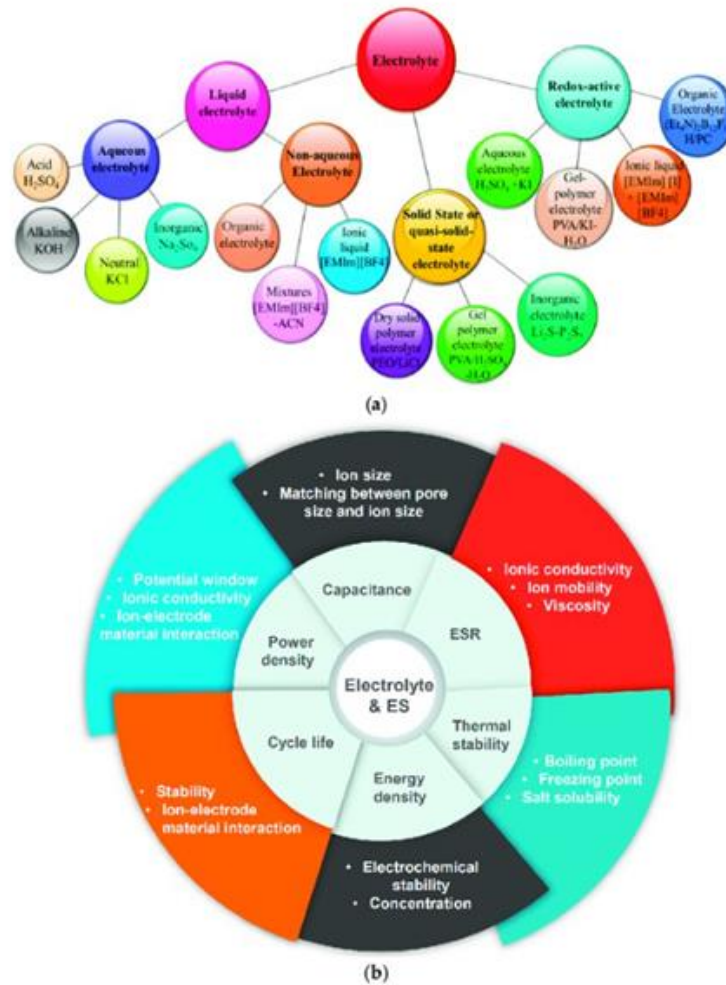
Figure 2.2.10. (a) Different types of electrolytes suitable for specific SC applications and (b) impact of the electrolyte on the performance of electrochemical SCs. (source: Tiwari, Santosh & Thakur, Anukul & De Adhikari, Amrita & Zhu, Yanqiu & Wang, Nannan. (2020). Current Research of Graphene-Based Nanocomposites and Their Application for Supercapacitors. 10. 2046. 10.3390/nano10102046.)
