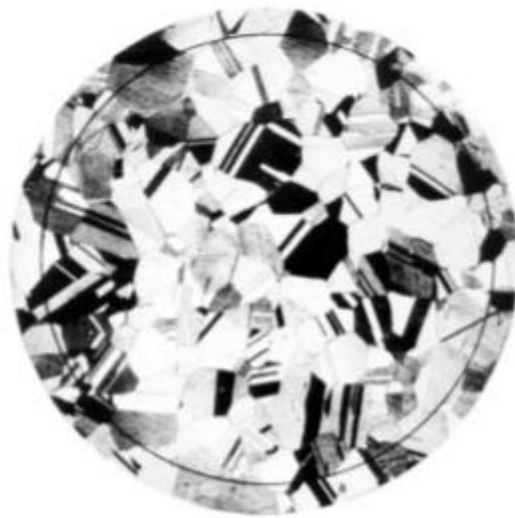
Fig. 2.3.9– example of twin grains (contrast Etchs) from plate III – Grain size 4 at 75X – image taken from ASTM E112. Source: [2.3.6] ASTM E112 – Standard Test methods for Determining Average Grain size
