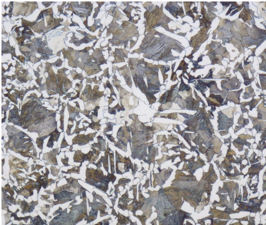
Fig. 3.5.5 – Detail of a medium carbon steel type C45 (C = 0.45 % wt) – Pearlite and ferrite isles. Etchant: Nital 2%. Source: IIS Laboratory
