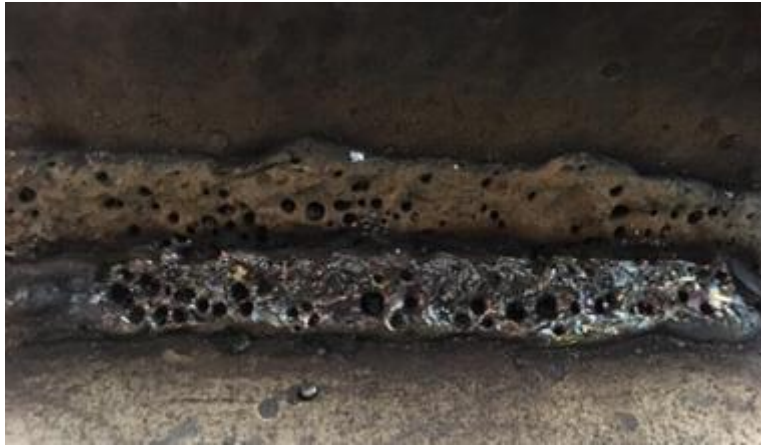
Fig. 3.2.27: Porosity. Source: https://www.mechanicwiz.com/porosity-in-welding/
