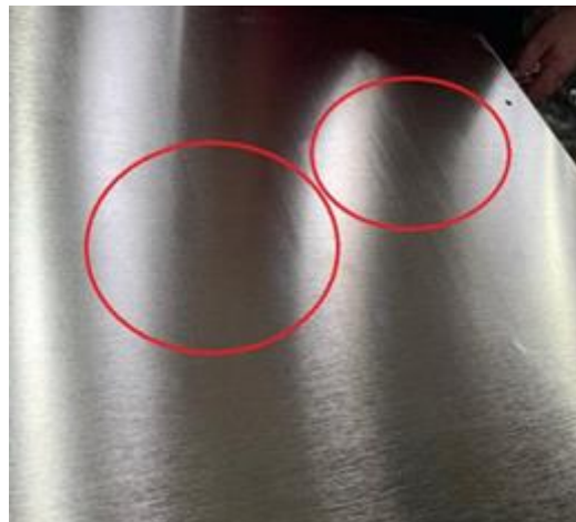
Figure 2.2.14. Uneven polishing on stainless steel sheet (source: AzOm)
