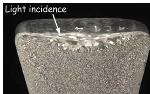
Fig. 2.1.41 Grain Boundary Assessment after Chemical Polishing for Stainless Steel [2.1.17]
