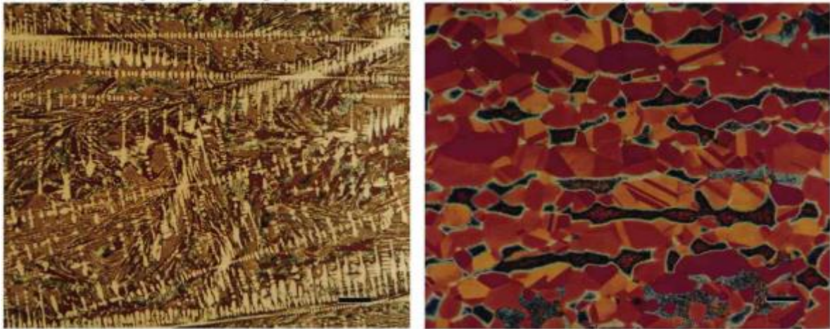
Fig. 2.1.31 and 2.1.32: Cementite in the chill cast surface of gray iron etched with Beraha's selenic acid reagent for cast iron (left) and twinned FCC alpha phase and beta phase (mottled and outlined) in Cu-40% Zn revealed using Beraha's selenic acid reagent for copper alloys. Magnification bars are 50 and 20 \mu\text{m} long, respectively [2.1.14].
