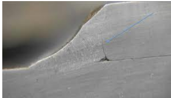
Fig. 3.2.29: Lack of fusion. Source: https://www.onestopndt.com/ndt-articles/what-is-lack-of-fusion-in-welds
