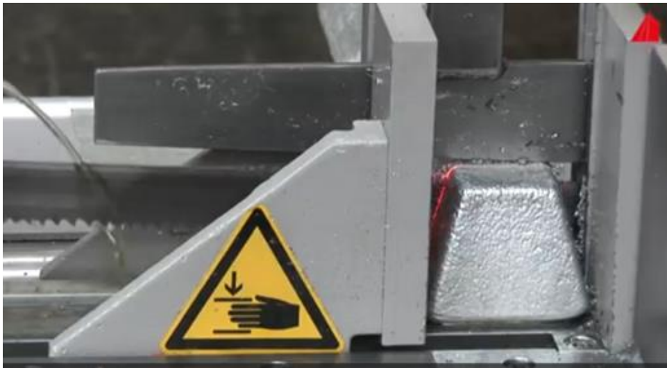
Figure 3.7.1. Mechanical cutting under water cooling
