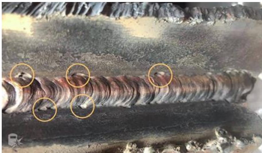
Fig. 3.2.31: Undercuts. Source: https://weldguru.com/undercut-in-welding/
