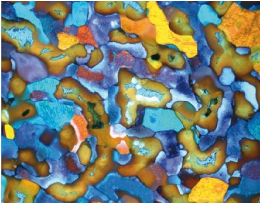
Figure 2.2.67. Concentration differences in a bronze wire (K) (source: Leica Microsystems)
