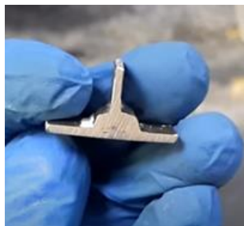
Figure 2.2.33. Preparation of the sample for colour etching (source: Vac Aero Coloured Metallography)
