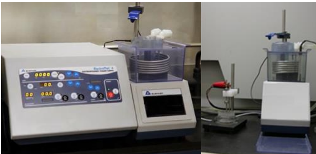
Figure 2.2.4. Equipment for electrolytic polisher with the electrolytic cell uncover (source: American Buehler Instrument Co., Ltd.)
